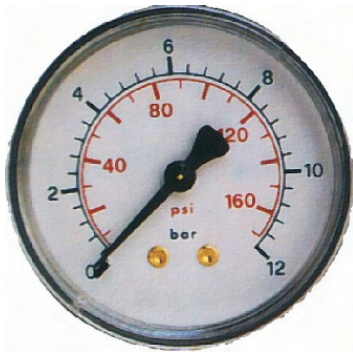
M C 50...: Ø 50 Axial pressure gauge ( available scale in bar: 4, 6,10,12,16 Bar ) 1/4" GAS connection- Back entry - Copper tubular spring – Sn-Ag welding - Working temperature: -20°C / +80°C – box: black plastic
