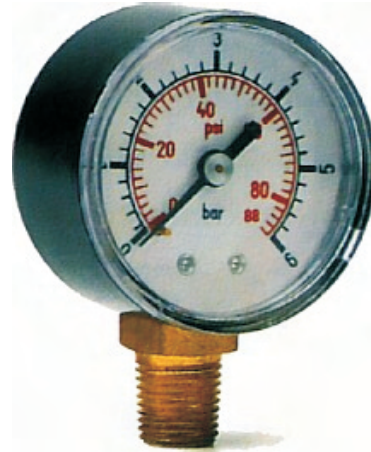
M R 63...Radial pressure gauge Ø 63 ( available scale in bar: 4,6,10,12,16 Bar ) 1/4" GAS connection- Bottom entry - Copper tubular spring – Sn-Ag welding Working temperature: -20°C / +80°C – box: black plastic
