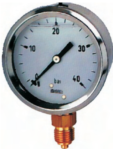
M GX ... : Pressure gauge with glycerine Ø 50., 63 or 100 ( available scales in bar: 4, 6 ,10 ,12,16, 20 ,25,40 e 100 Bar )1/4" GAS connection ( 1/2" connection for r Ø 100) Bottom entry (M GX ...R) or back entry ( M GX C ) – Working temperature: -10°C /+ 80°C STAINLESS STEEL CONSTRUCTION
