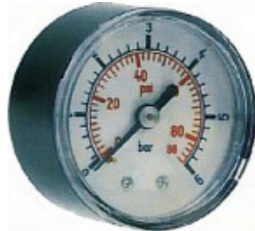
M R 63...Radial pressure gauge Ø 63 ( available scale in bar: 4,6,10,12,16 Bar ) 1/4" GAS connection- Bottom entry - Copper tubular spring – Sn-Ag welding Working temperature: -20°C / +80°C – box: black plastic
