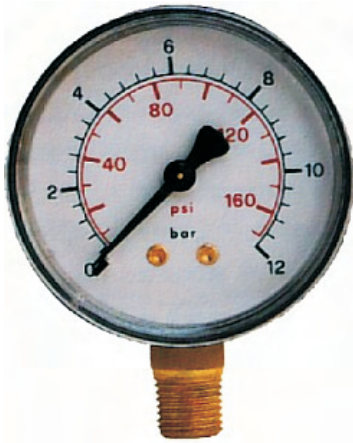
M R 50...: Radial pressure gauge Ø 50 ( available scale in bar: 4, 6,10,12,16 Bar ) 1/4" GAS connection- Bottom entry - Copper tubular spring – Sn-Ag welding - Working temperature: -20°C / +80°C – box: black plastic
